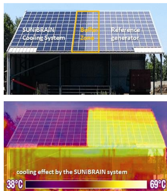
Figure 1: (Top) Test System consisting in 2 twin generators separated by a buffer zone. (Bottom) Thermographic image of the roof showing the cooling effect by the SUNiBRAIN system.
